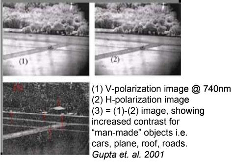
Figure 5 Enhancement of detection by differential polarisation imaging
