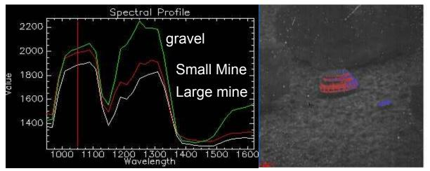
Figure 3 Spectral classification and detection of mines
